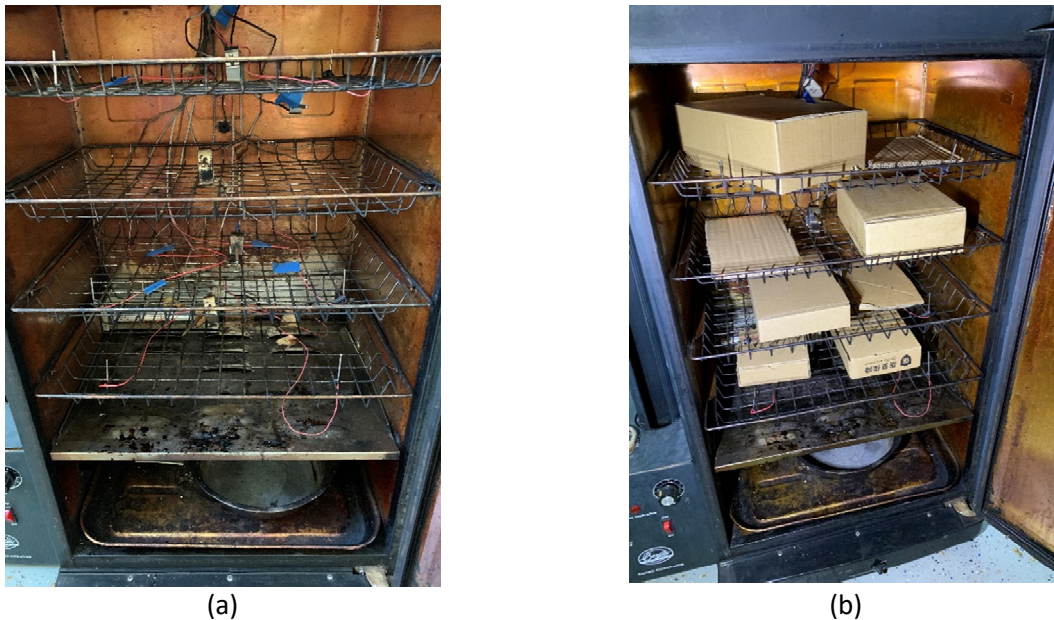
Figure 2. (a) Totally 18 temperature probes were installed on a 4-rack Bradley Original Smoker. (b) Different sized cardboard boxes were randomly arranged in the smoker to simulate the obstruction on the air flow by food placed in a smoker.
